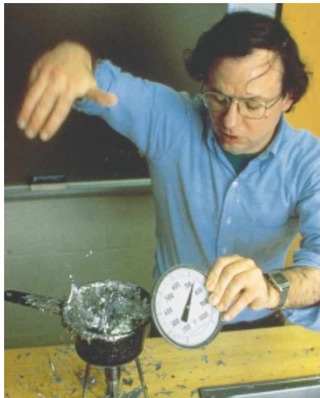
Fig. 5 Walker demonstrating the Leidenfrost effect with molten lead. He has just plunged his fingers into the lead, touching the bottom of the pan. The temperature of the lead is given in degrees Fahrenheit on the industrial thermometer.
