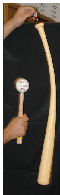
Fig. 2. A pulse created by a collision with the baseball hammer.
