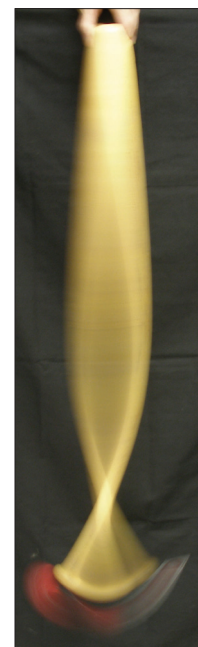
Fig. 3. The first normal mode or standing wave in the bat.
