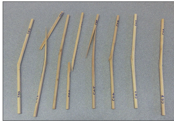
Fig. 5. The broken ash dowels. Note that only three of eight broke resulted in sharp edges.
