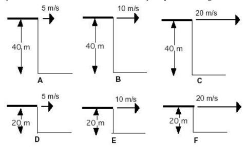
The vertical motion is independent of the horizontal motion. The vertical motion is freefall, so the time of fall just depends upon the height. So, A, B and C take the same time to fall as do D, E and F. A, B, and C take longer because the water has further to fall.
