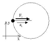
(a) The only force acting on the ball is the tension in the string (if gravity is ignored). Applying the Second Law.
