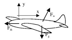
Using the free body diagram at the right and applying Newton's Second Law,
