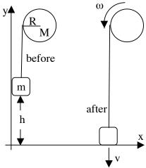
Initially, the kinetic energy is zero and the hanging mass has some gravitational potential energy,
