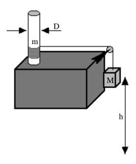
2. A device for measuring the rotational inertia I of an object is shown. The object (not shown but assume it is there) should be placed on top of a shaft of diameter D and mass m that has a string wrapped around it. The string is connected to a hanging mass M which falls a distance h in a time t. Find the equation for the rotational inertia of the object in terms of D, m, M, h, and t.
