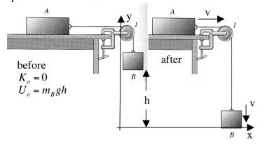
The final potential energy is zero, but the kinetic energy includes the motion of the masses and the pulley,
