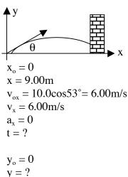
$v_{oy} = 10.0 \sin 53^\circ = 8.00 \text{m/s}$
