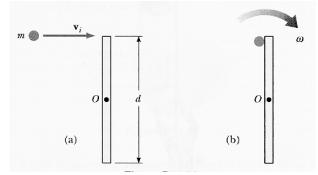
The final angular momentum is due to the motion of the stick and the clay,  $L = I\omega + \frac{d}{2}mv$ .
