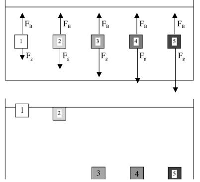
Since the blocks are all the same size, they displace the same amount of water. By Archimedes Principle, they must have the same buoyant force. Since the denser blocks have more mass, they have a greater gravitational force.
