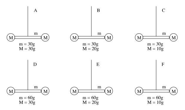
These are torsional pendulums. The angular frequency of a torsional pendulum is  $\omega = \sqrt{\frac{\kappa}{I}}$ .
