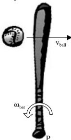
8. A  $0.900\pm0.001$ kg baseball bat is  $85.0\pm0.2$ cm long and its center of mass is  $55.0\pm0.2$ cm from the knob end. When held at the knob end and allowed to oscillate, it is found to have a period of  $1.60\pm0.05$ s. Find the rotational inertia of the bat about the knob end and find the uncertainty in this value.
