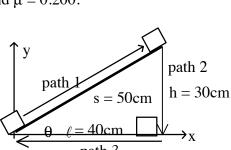
Since the work done by the frictional force around the closed path is not zero, the force of friction is a non-conservative force.
