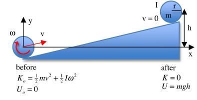
$$\Delta U + \Delta K = 0 \Rightarrow \left[ mgh - 0 \right] + \left[ 0 - \left( \frac{1}{2} mv^2 + \frac{1}{2} I\omega^2 \right) \right] \Rightarrow mgh = \frac{1}{2} mv^2 + \frac{1}{2} I\omega^2 .$$
