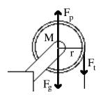
Note that the only force causing a torque about the center of the pulley is the tension. Applying the Second Law for Rotation,
