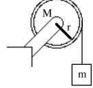
It is best to attack these types of problems by looking at separate parts of the system. Considering just the forces on the hanging weight and applying Newton's Second Law,
