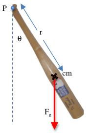
Angular Frequency of a Physical Pendulum
