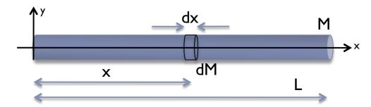
A uniform stick has a length L and a mass M. It can be broken down into small pieces of mass dM of length dx as shown above.
