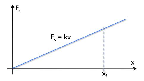
Consider finding the work is done to stretch the spring from zero to  $x_f$ . The graph above shows the force as it changes with the position.
