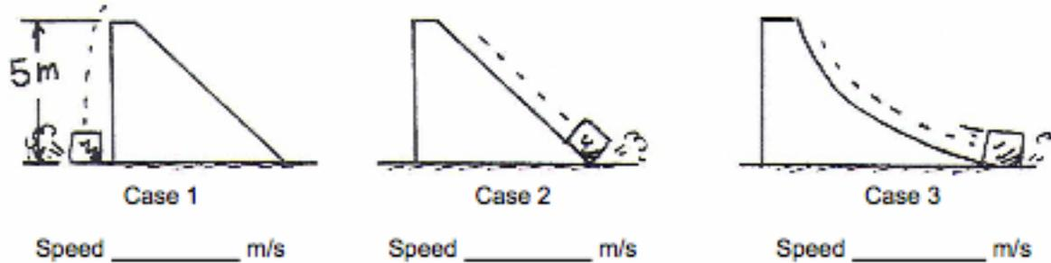
Above are three situations involving ramps of the same height. In case 1, a 1.0kg block is dropped from the top of the ramp. In the other two cases, the 1.0kg block slides down the ramp. The goal is to find the speed of the block at the bottom. Fill in the tables below:
