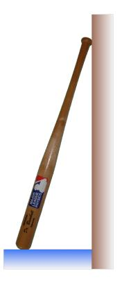
Example 6: An I.0kg baseball bat has a center of mass 60cm from the handle. It is 90cm long and leans against a smooth wall making a 53° with the floor. Find the minimum coefficient of friction required to keep the bat from slipping.
