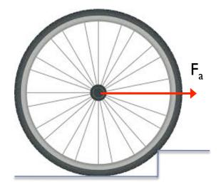
Example 2: A 1.00kg bicycle wheel with a radius of 22.0cm comes up against a curb 6.00cm high. The bike exerts a horizontal force on the axle. Find the size of the force exerted by the axle if the wheel is to go over the curb.
