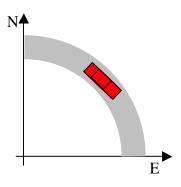
3. A car rounds a curve of radius 25.0m that is banked at 20.0°. The coefficient of static friction between the road and the car is 0.520. Find the maximum velocity that a car can have and make this turn.
