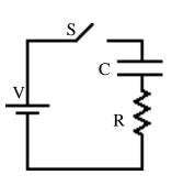
The charge on the capacitor varies with time according to,
