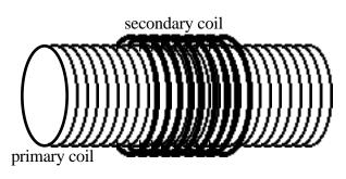
Case 1: The battery was recently connected. The current in the primary is in the direction shown and growing.
