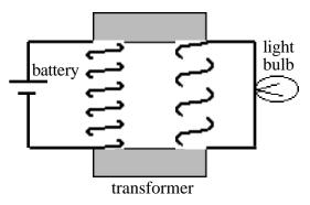
secondary coil with the light bulb. According to Faraday's Law the changing field induces a voltage that lights the bulb.
