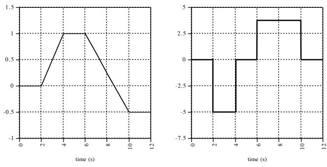
(a) Using Faraday's Law the induced voltage is,  $\oint \vec{E} \cdot d\vec{s} = -\frac{d\Phi_B}{dt} \Rightarrow V = -N\frac{d\Phi_B}{dt}$ .
