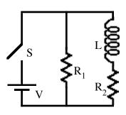
When the switch is closed the voltage across both legs of the circuit must equal the battery voltage by the loop theorem. At all times then the voltage on  $R_1$  must equal V and the voltage on L and  $R_2$  must sum to V.
