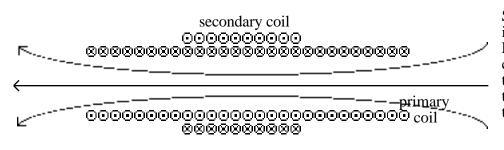
Since the field to the left is increasing, according to Faraday's Law and Lenz's Rule, the secondary coil will produce a field that fights the increase. Therefor, the field due to the secondary must be opposite to the field of the primary.
