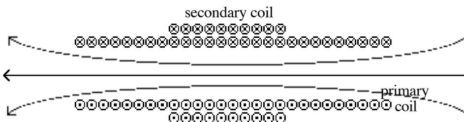
Since the field to the left is decreasing, according to Faraday's Law and Lenz's Rule, the secondary coil will produce a field that fights the decrease. Therefore, the field due to the secondary must be in the same direction as the field of the primary.
