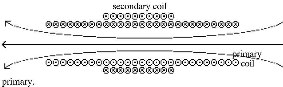
Since the field to the left is increasing, according to Faraday's Law and Lenz's Rule, the secondary coil will produce a field that fights the increase. Therefore, the field due to the secondary must be opposite to the field of the primary.
