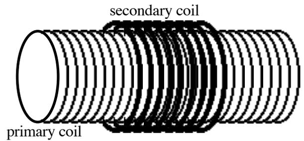
Case 1: The battery was recently connected. The current in the primary is in the direction shown and growing.
