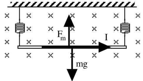
According to the right hand rule, the current must be moving toward the right in order to feel an upward force.
