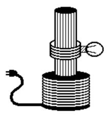
8. A 1000 turn coil with a radius of 6.00cm spins with a period of 50.0ms. The axis of the coil is horizontal and points eastward, while the earth's magnetic field of  $52.0\mu T$  points northward at  $62^{\circ}$  below horizontal. Find the peak voltage induced in the coil.
