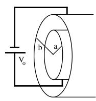
Applying Gauss's Law to an imaginary cylinder with a radius r between a and b. Since the cylinders are long, symmetry requires the field to be constant over this Gaussian cylinder as it must point radially outward. Therefor,
