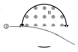
(a)As the electrons are accelerated they lose 3000eV of potential energy. By the Law of Conservation of Energy they gain 3000eV of kinetic energy,
