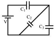
Since  $C_3$  is in parallel with  $C_2$ , they both have the same potential difference. Now, the charge on  $C_2$  can be found,
