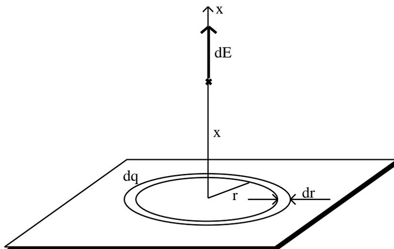
From example 10 we know the field due to a ring of charge, so break the plane up into an infinite number of rings with charge,  $dq$ , radius,  $r$ , and thickness  $dr$ . Each ring creates a field,  $dE = k \frac{x dq}{(r^2 + x^2)^{3/2}}$ .
