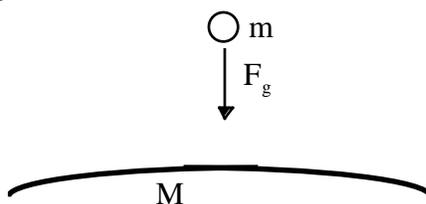
In this view, Earth creates a force on the mass  $m$ . This is "insane." Earth isn't even touching the mass. So we introduce the idea of a gravitational field.
