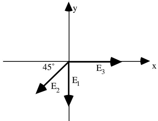
Using the field due to a point charge,  $\vec{E} = k \frac{q}{r^2} \hat{r}$ , find the magnitude of each field vector.
