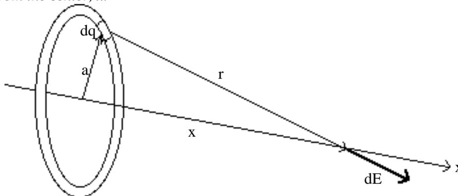
Using the field due to the point charge  $dq$ ,  $d\vec{E} = k \frac{dq}{r^2} \hat{r}$ . By the symmetry of this problem the field will only point in the x-direction so we only have to worry about the x-components,
