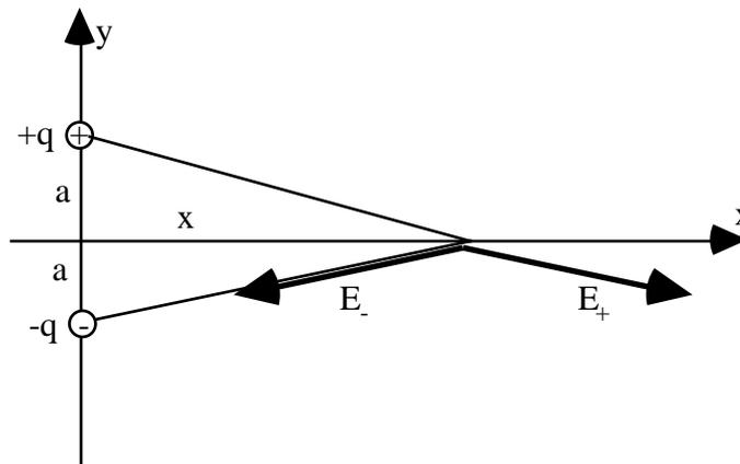
Use the field due to a point charge,  $\vec{E} = k \frac{q}{r^2} \hat{r}$ , to find the magnitude of both field vectors. Notice
