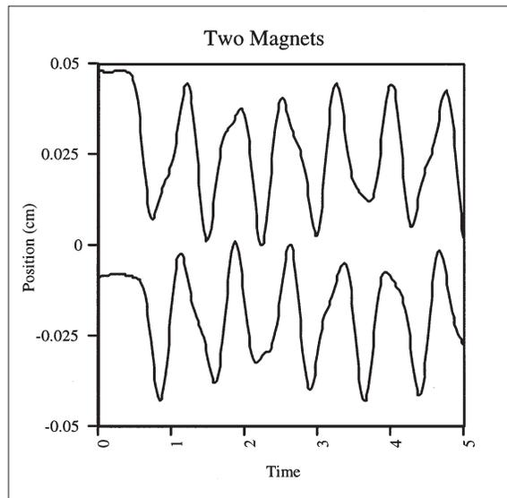
**Fig. 4. Position-vs-time graph for two colliding magnets.**
