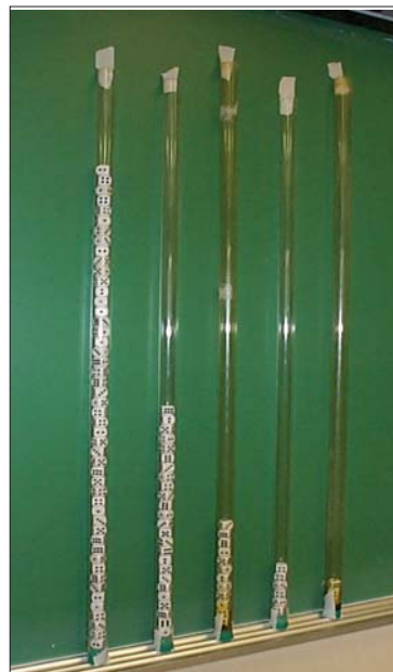
Fig. 1. The tubes, mounted against the blackboard, filled with dice using a 50% probability of decay.
