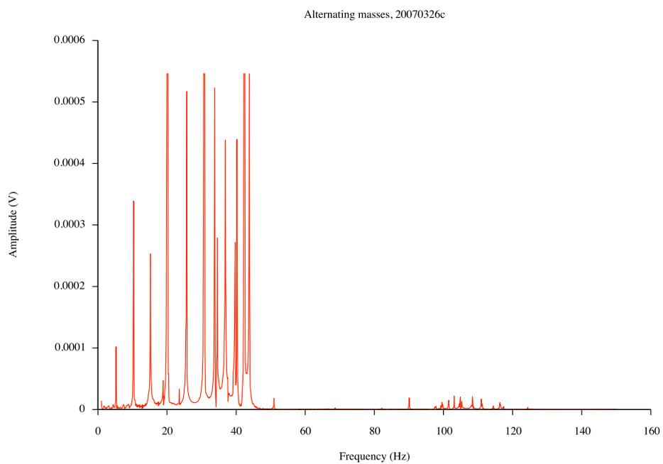
Figure 4: Frequency response of the “one-dimensional crystal”. Note that the frequency scale is the *driving* frequency to the excitation coil: the frequency of the wire is twice this value.
