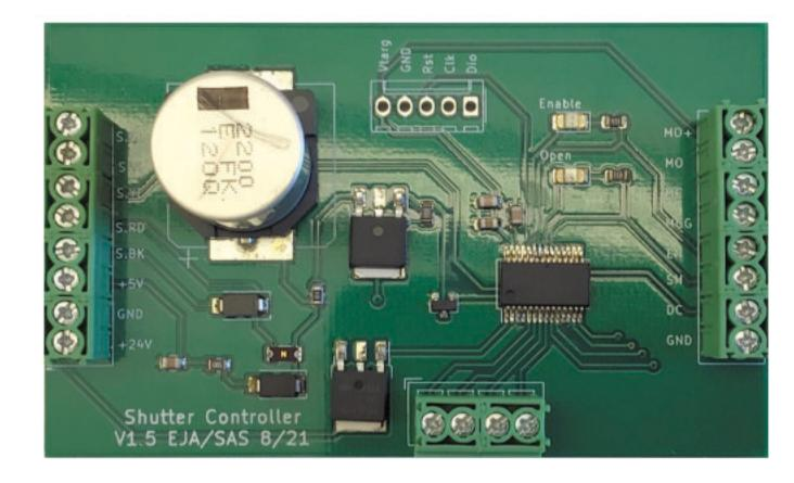
The completed board has connections for the 24V and 5V supplies, the safety interlock(s), additional digital indicator lines for the computer controlling the experiment, and all of the shutter wiring.
