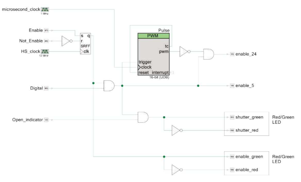
Any microcontroller could provide the signals to the voltage-control circuit. We chose to use a PSoC because it allows hardware-based digital logic for implementation of any interlock safety features that may be desired. Instead of a microcontroller program running continuously to check the state of the interlock and computer signals, the logic shown above responds almost instantly to any changes in the input.
