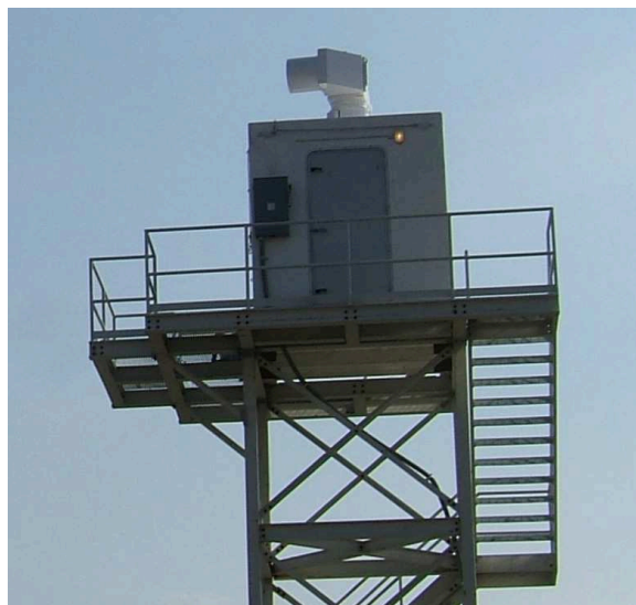
Figure 4. The first REAL “v2” created through a tech-transfer licensing agreement between a commercial firm and NCAR. The unit operates continuously (except for flashlamp changes every 2 weeks) and unattended for the automatic detection and tracking of aerosol plumes in Washington DC.
