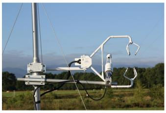
Above left: Photo of a tower supporting atmospheric flux measuring instrumentation. Right: an ultrasonic anemometer and a LICOR 7500 open path gas analyzer. Fluxes are determined by a measurement technique known as *eddy covariance*.
